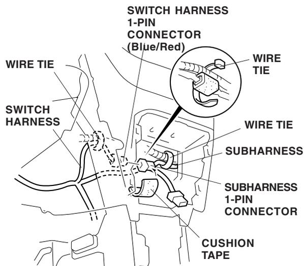
51. Secure the subharness and switch harness to the vehicle harness with two wire ties in the areas shown.
