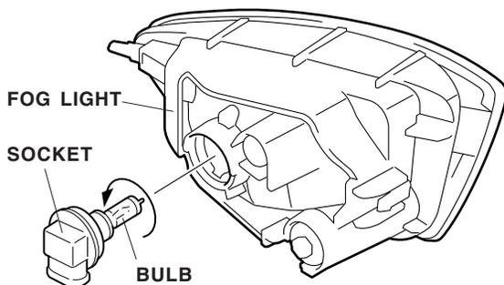
4. Install the new bulb and socket into the fog light.
