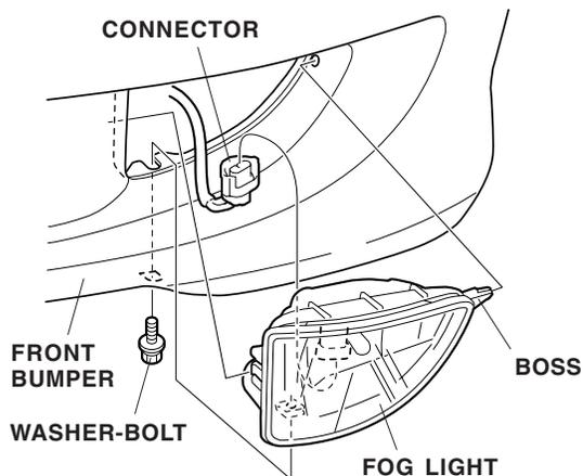
3. Remove the bulb along with the socket.
