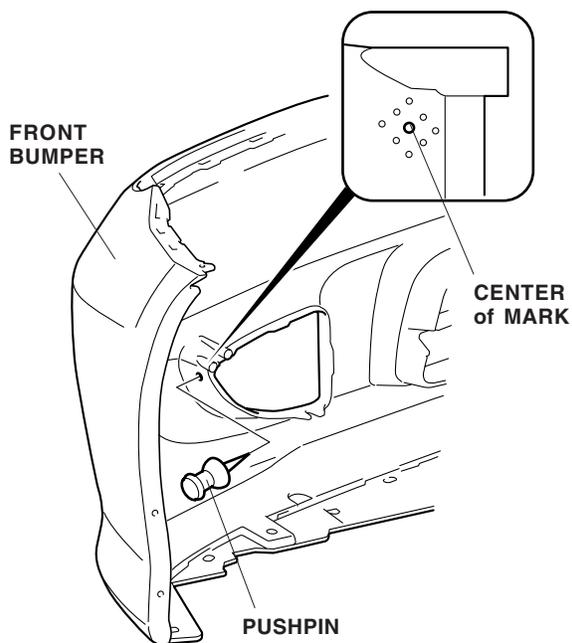
8. While wearing eye protection, drill an 8 mm hole through the hole you just made. First drill with a 3 mm drill bit, then with a 6 mm drill bit, and finish with an 8 mm drill bit. Remove any burrs from the edge of the hole.
