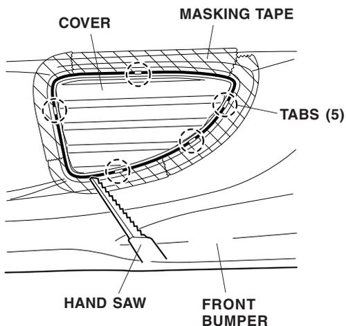
5. Wearing gloves, remove the cover from the left side of the front bumper by cutting the five tabs with a hand saw.
