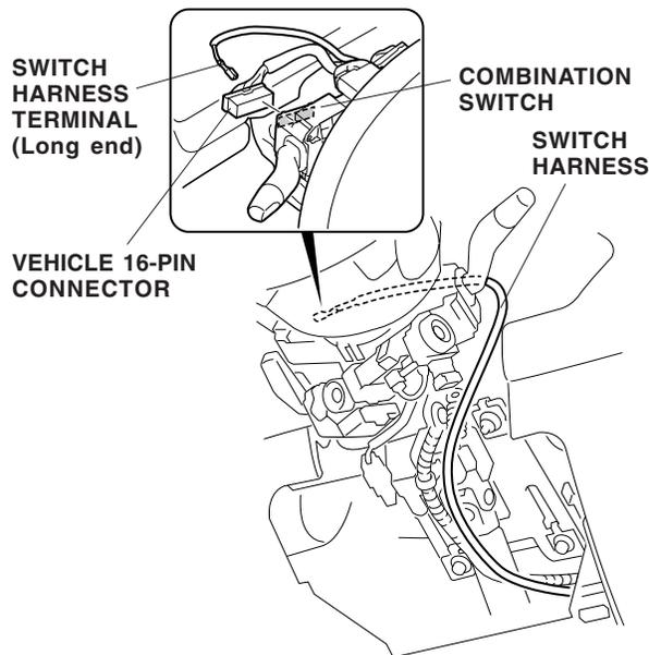
56. On the left side of the combination switch, unplug the vehicle 16-pin connector.
