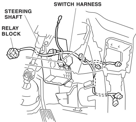
43. Attach the relay bracket to the steering hanger beam using the washer-bolt.
