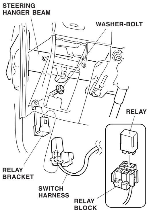
44. Plug the relay into the relay block, then attach the relay block to the relay bracket.
