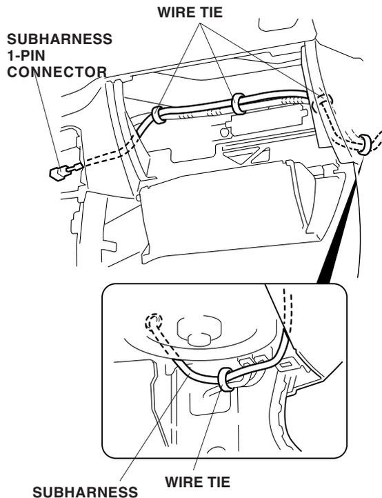
42. Get the switch harness. Route the switch harness under the dash, and over the steering shaft and brake position switch harness.
