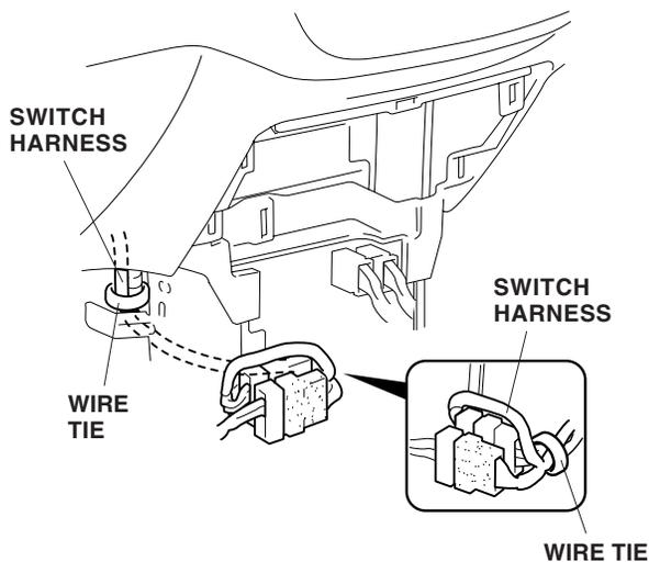
50. Plug the subharness 1-pin connector (routed in step 43) into the switch harness 1-pin connector (blue/red), then wrap one cushion tape around the connectors. Secure the connector to the vehicle harness using one wire tie.
