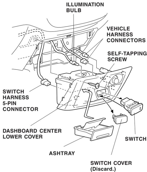
53. Plug the switch harness 6-pin connector into the fog light switch, then install the fog light switch into the center lower trim.
