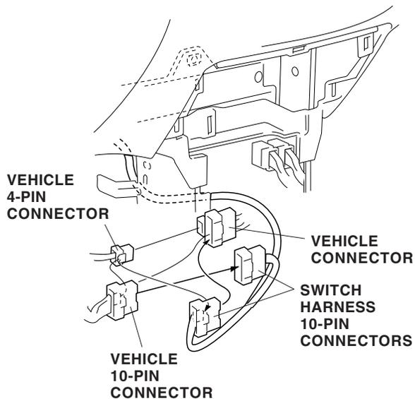
49. Secure the switch harness to the vehicle harness with two wire ties in the areas shown.
