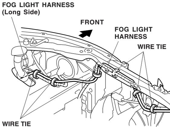
**Without Air Conditioner:** Secure the fog light harness to the vehicle harness with three wire ties, then secure the the fog light harness to the front and side frame using three wire ties with clips in the areas shown.
