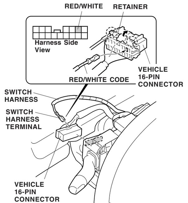
58. Reconnect the vehicle 16-pin connector.
