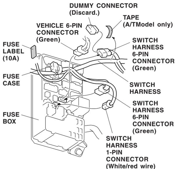
46. Plug the switch harness 1-pin connector (white/red wire) into the fuse box in the location shown.
