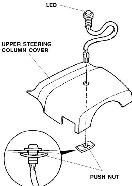
11. Carefully push the LED terminals into the 2-pin connector from the kit.
