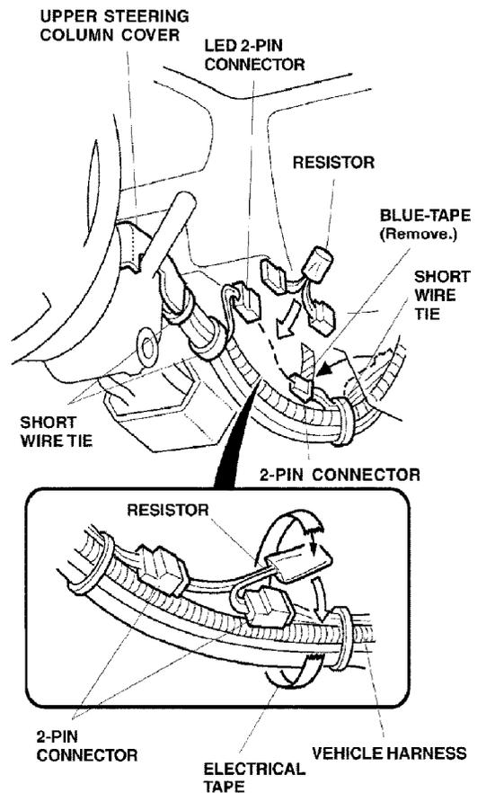
27. Tape the resistor to the vehicle harness using electrical tape. Secure the LED harness to the vehicle harness with the three short wire ties in the areas shown.
