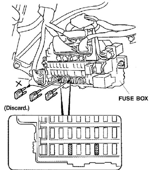
21. Push the two fuses from the kit into the number 3 and number 6 slots in the fuse box.
