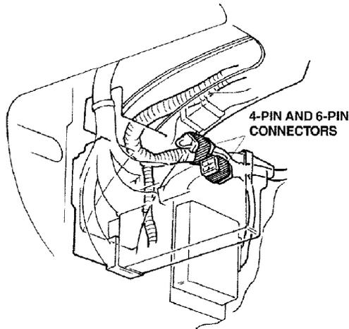
24. Locate the 4-pin connector blue-taped to the vehicle harness above the fuse box, and remove the tape to free the connector. Plug the 4-pin relay into the 4-pin connector you just freed, then secure the relay to the vehicle harness with the wire tie.
