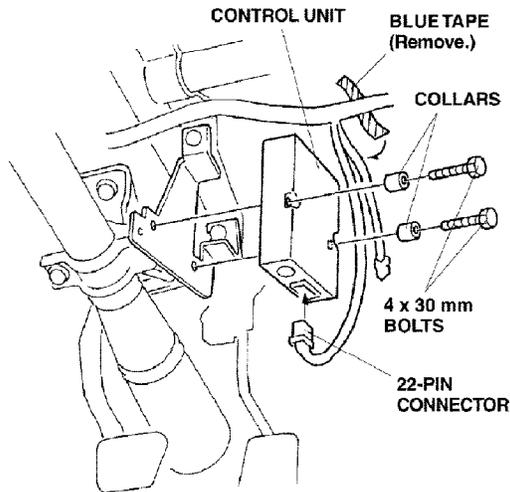
19. Locate the 22-pin connector blue-taped to the vehicle harness, and remove the blue tape to free the connector. Plug the 22-pin connector you just freed into the control unit.
