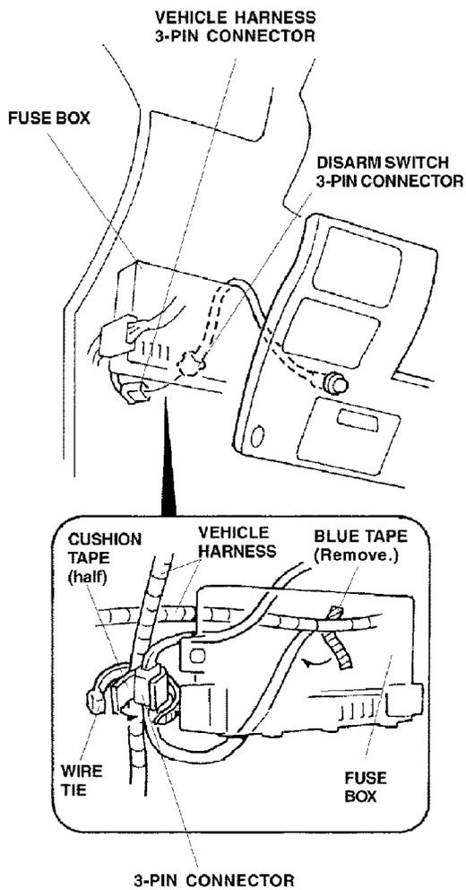
30. Wrap half of a cushion tape around the 3-pin connectors, then secure them to the vehicle harness with one wire tie as shown.
