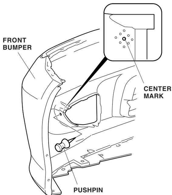
8. While wearing eye protection, drill an 8 mm hole through the hole you just made. First drill with a 3 mm drill bit, then with a 6 mm drill bit, and finish with an 8 mm drill bit. Remove any burrs from the edge of the hole.
