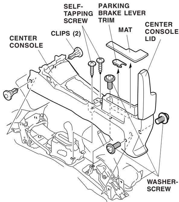
40. Remove the parking brake lever trim, and remove the center console (two self-tapping screws, three washer-screws and two clips).
