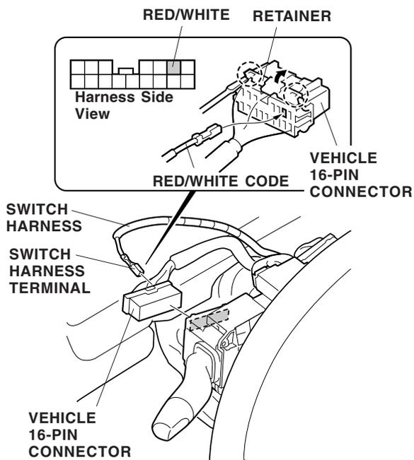
60. Reconnect the vehicle 16-pin connector.
