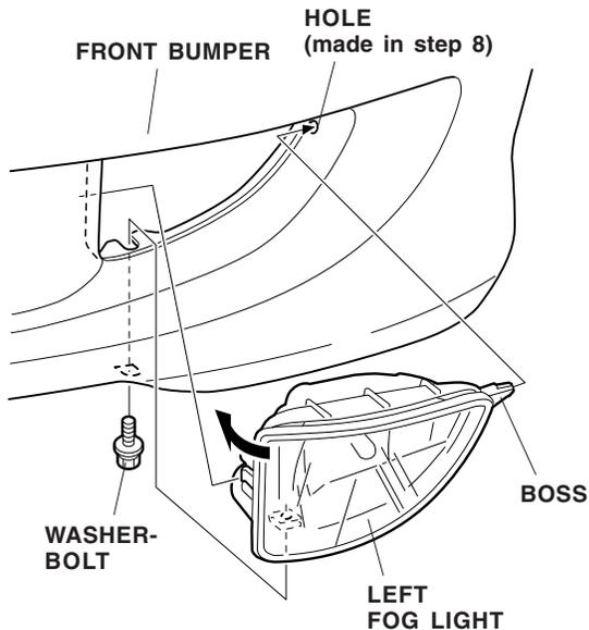
24. Under the front bumper, install the washer-bolt to secure the left fog light to the front bumper.
