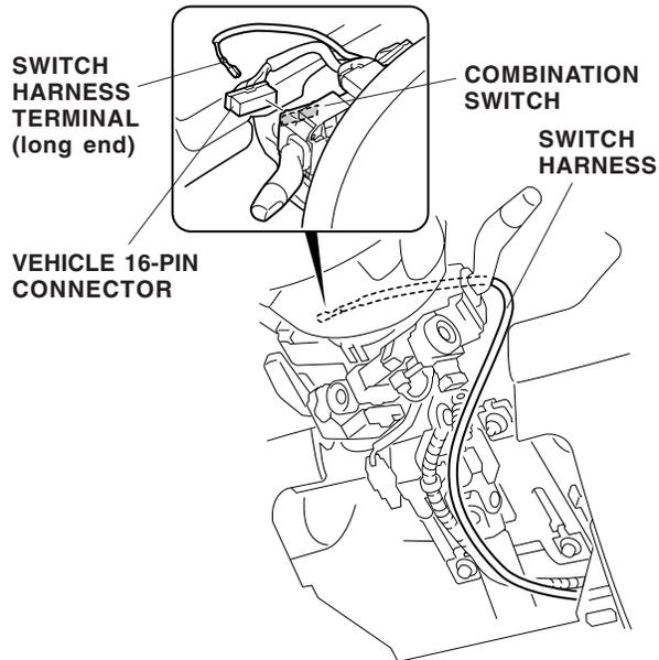
58. On the left side of the combination switch, unplug the vehicle 16-pin connector.
