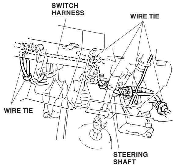
63. Check that all wire harnesses are routed properly and all connectors are plugged in.
