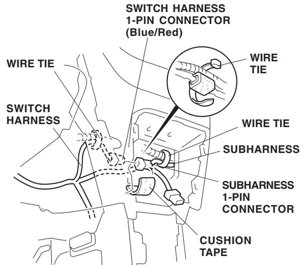
53. Secure the subharness and switch harness to the vehicle harness with two wire ties in the areas shown.
