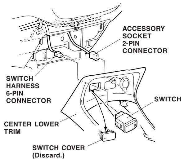
55. Plug the switch harness 6-pin connector into the fog light switch, then install the fog light switch into the center lower trim.
