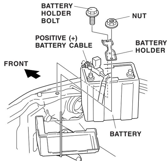
11. Remove the battery holder bolt and nut, then remove the battery holder.
