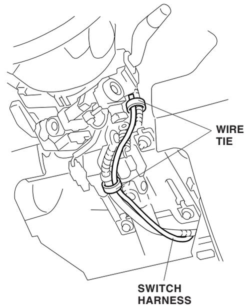
62. Under the dash, secure the switch harness to the vehicle harness with six wire ties in the areas shown.
