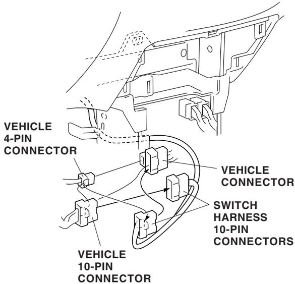
51. Secure the switch harness to the vehicle harness with two wire ties in the areas shown.
